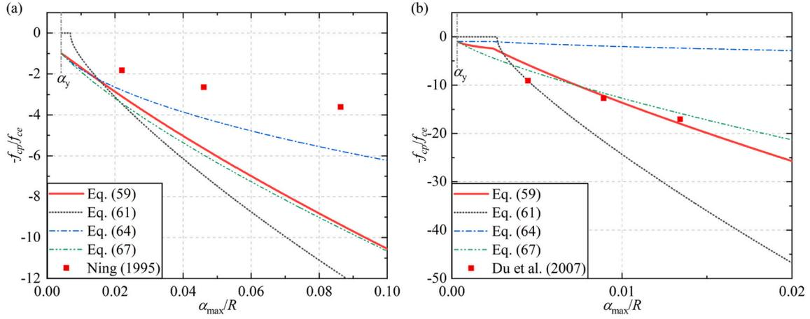
**Fig. 7.** Comparisons of maximum pull-off force  $f_{cp}$  predicted by different methods with (a) Ning (1995) and (b) Du et al. (2007) under different maximum normal overlaps  $\alpha_{max}$  (i.e. the overlap at which the unloading commences).
