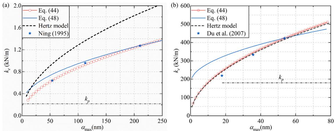
**Fig. 6.** Comparisons of stiffness  $k_e$  predicted by different methods with (a) Ning (1995) and (b) Du et al. (2007) under different maximum normal overlaps  $\alpha_{\max}$  (i.e. the overlap at which the unloading commences).
