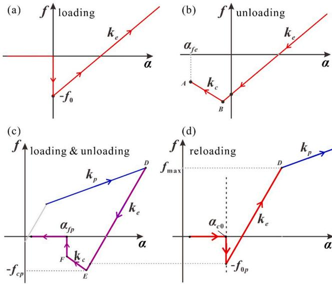
Fig. 2. Schematic diagram of the normal force  $f$ -overlap  $\alpha$  relationship in the loading/unloading and reloading processes for the contact: (a-b)-without plastic deformation ( $f_{\max} < f_y$ ), where  $k_e$  is a constant and corresponds to the lower limit of  $k_e$ , and it is assigned as  $k_{el}$  for convenience; (c-d)-with plastic deformation ( $f_{\max} > f_y$ ), where  $k_e$  varies with  $\alpha_{\max}$ .
