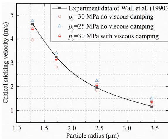
**Fig. 10.** Comparisons of critical sticking velocity  $V_{ys}$  predicted by this work with the experimental data of Wall et al. (1990).
