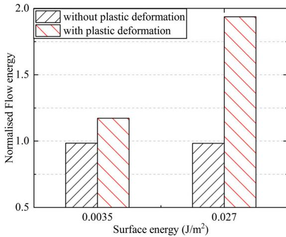
**Fig. 12.** Flow energy of cohesive powder in FT4 rheometer predicted by the linear elasto-plastic and adhesive contact model: without and with considering plastic deformation; the flow energy is calculated at the penetration depth of 10 mm and normalised by the ones predicted by the DEM simulation using Hertz-Mindlin model with JKR theory.
