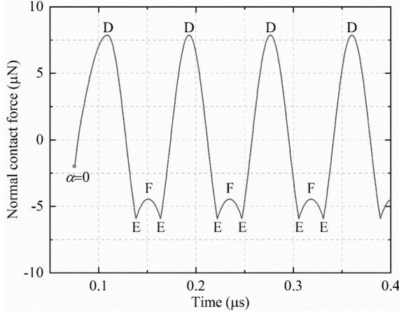
Fig. 3. Example of the oscillation of normal contact force with time if there is no viscous damping after yielding.
