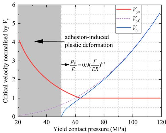
**Fig. 9.** Variation of critical velocity with yield contact pressure, where the velocity is normalised by adhesive sticking velocity  $V_s$  predicted by JKR theory;  $V_{ys}$  is the critical sticking velocity considering both cohesion and plastic deformation;  $V_{y0}$  (not considering cohesion effect) and  $V_y$  (considering cohesion effect) are the yielding velocity, above which the contact could be yielded.
