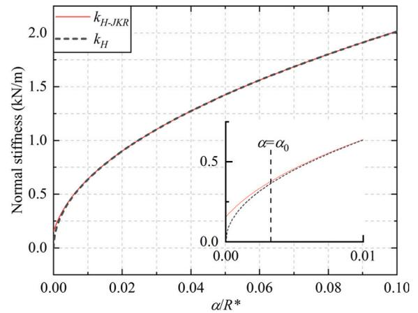
**Fig. 13.** Variation of normal stiffness with normal overlap in Hertz model and Hertz-JKR model for the case with  $R^* = 2.45 \mu\text{m}$ ,  $E^* = 1.3 \text{ GPa}$  and  $\Gamma = 0.2 \text{ J/m}^2$ .
