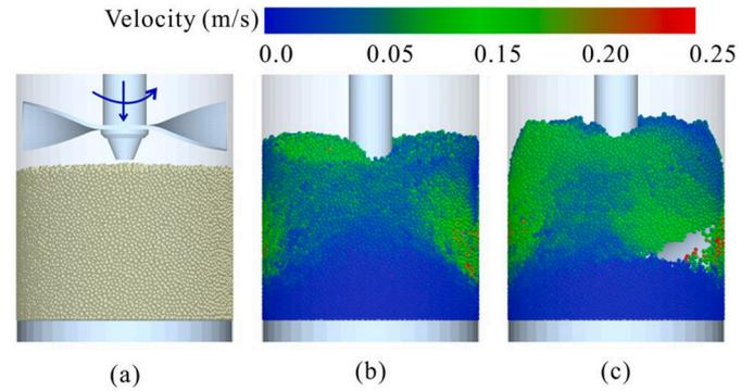
**Fig. 11.** Snapshots of particle flow ( $\Gamma = 27$  mJ/m<sup>2</sup>) in FT4 rheometer: (a) initial particle bed with blade rotating anti-clockwise while penetrating down; (b) reference case considering only cohesion (using Hertz model with JKR theory); (c) considering both cohesion and plastic deformation (using the linear elasto-plastic and adhesive contact model developed in this work); (b) and (c) are at both the same penetration depth (i.e. time) and viewpoint.
