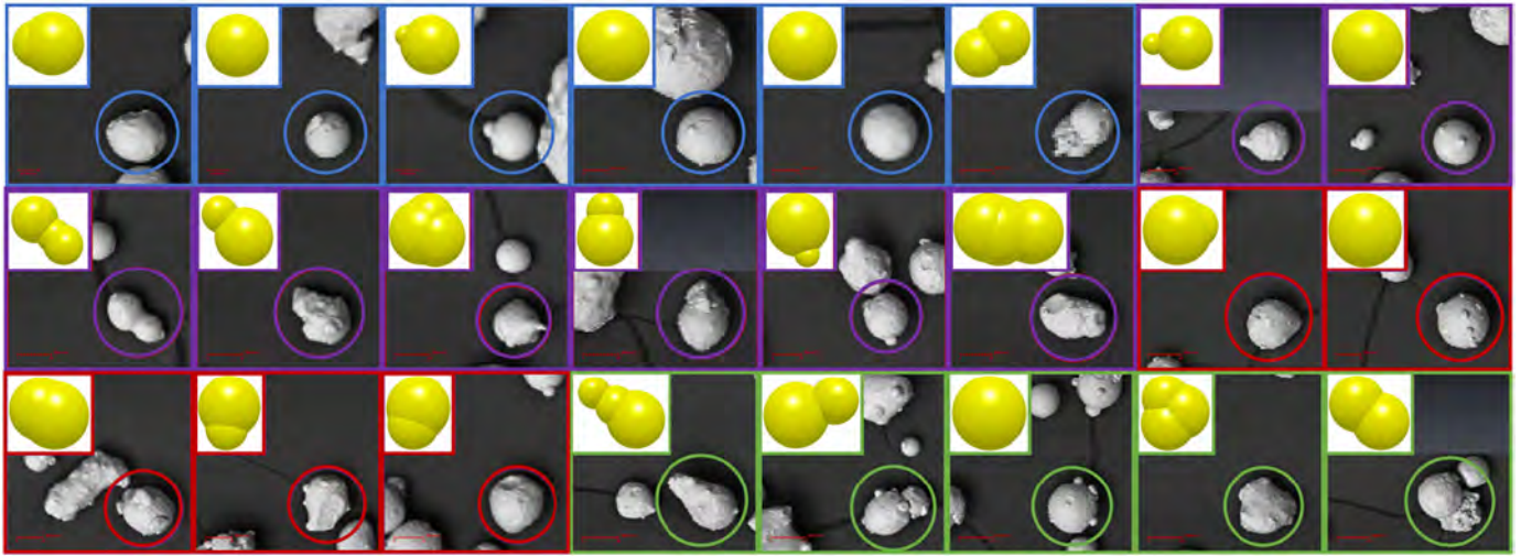
Fig. 3. Particle shapes used in DEM simulations; each size and shape class are represented by a colour circle, as shape varies with size; six blue circles (15–25 \mu\text{m} ), eight purple circles (25–35 \mu\text{m} ), five red circles (35–45 \mu\text{m} ), and five green circles (45–55 \mu\text{m} ).
